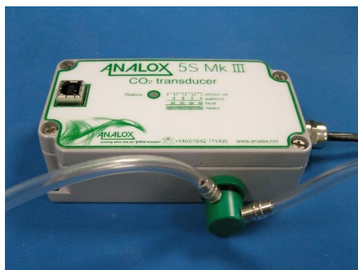
Single port sensor (% ranges) monitoring a remote atmosphere via a sample line.
