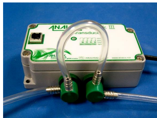
Dual port sensor (ppm ranges) monitoring a remote atmosphere via a sample line
