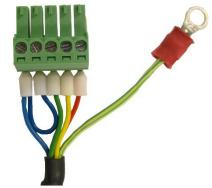
Use of the screen will depend on the particular installation. It is best connected to a clean Earth to form a shield around the sensor cable. Note that it is not recommended for the screen to be connected to the negative supply line.
