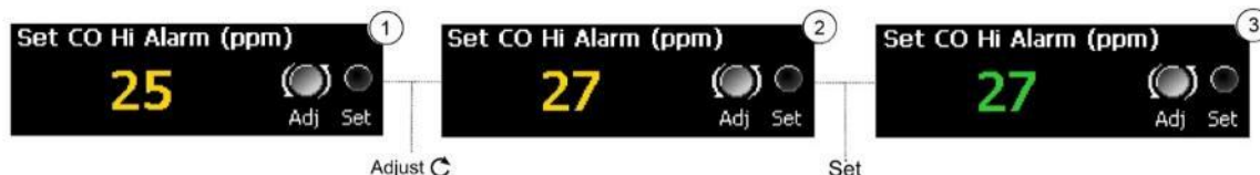
Figure 22 Example of alarm set-point adjustment
