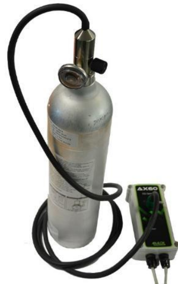
Step 4] Fit the regulator to the CO 2 check gas bottle
