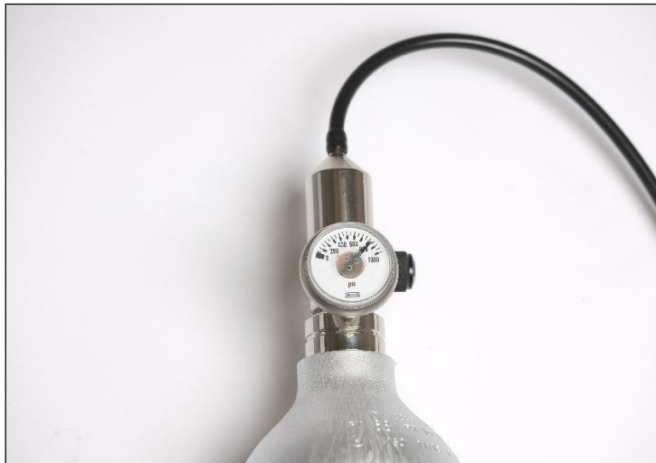
Figure 26 Flow Regulator Fitted to Calibration Bottle
