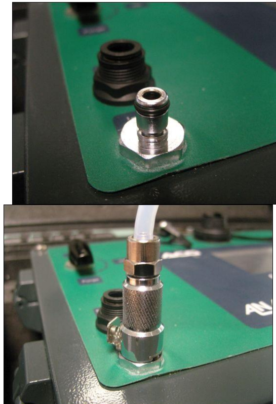
Figure 27 Connecting Calibration Fitting to ACG+ Calibration Port
