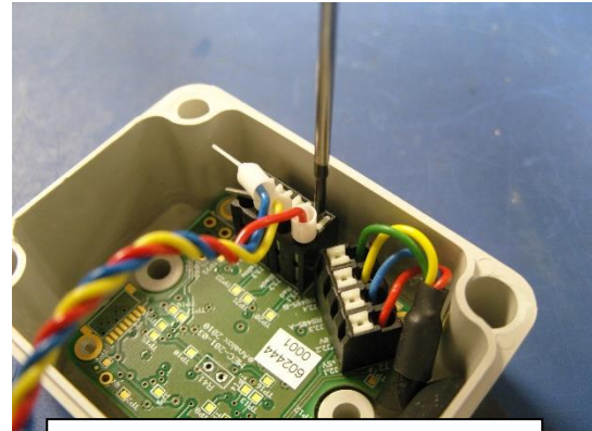
While still pressing down on the terminal clamp button insert the bootlaced wire into the terminal clamp as shown.
