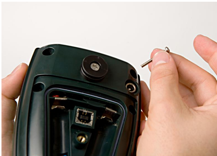
Figure 27 Replace the sensor cap and secure the screws
