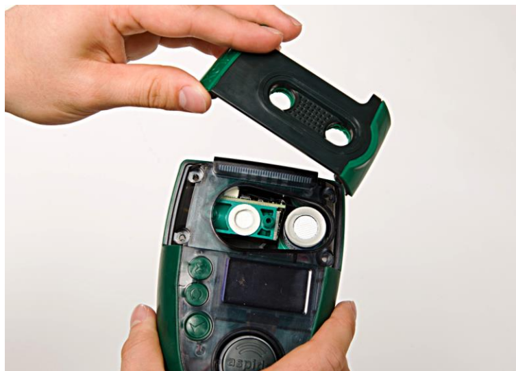
Figure 17 Remove the sensor cap
