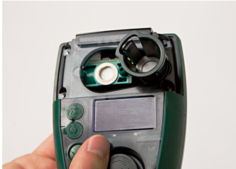
Figure 20 Correct extraction tool position
