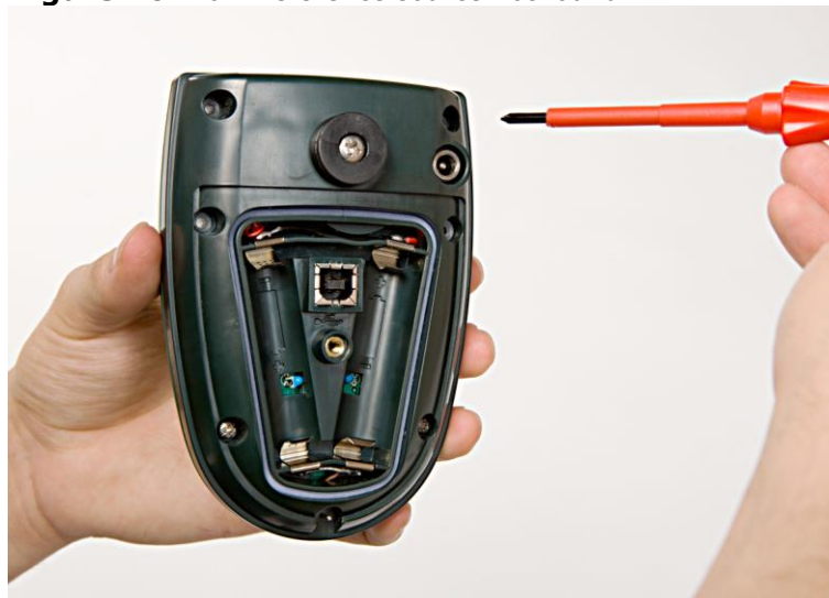
Figure 16 Remove the sensor cap screws
