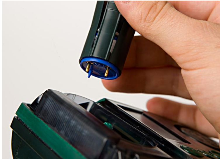
Figure 22 Removing the oxygen sensor
