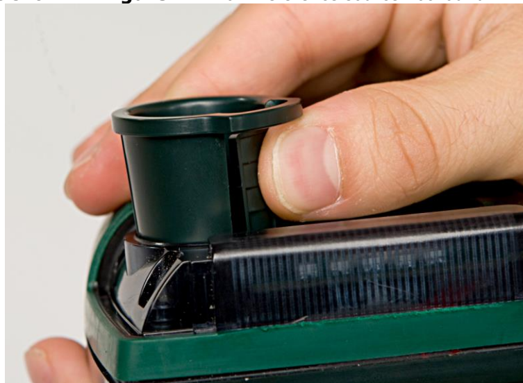
Figure 21 Squeeze the extraction tool
