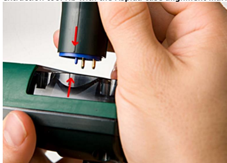
Figure 25 Align the new sensor with the Aspida device
