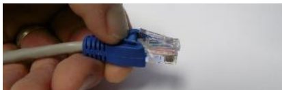
Pull boot back to access lock clip
