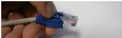
Pull boot back to access lock clip
