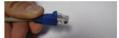
Slide boot back over lock clip
