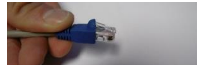
Slide boot back over lock clip
