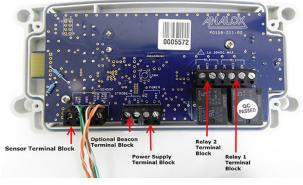
The Central Display's terminal blocks must be connected to the power supply, beacon and relays (the Sensor terminal block has a cable already fitted).
